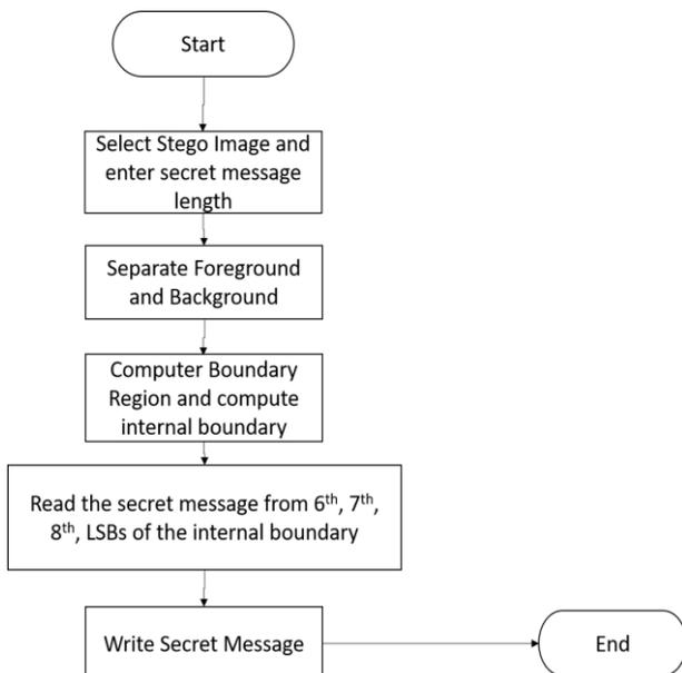
**Fig.3 Workflow of Extracting algorithm**
