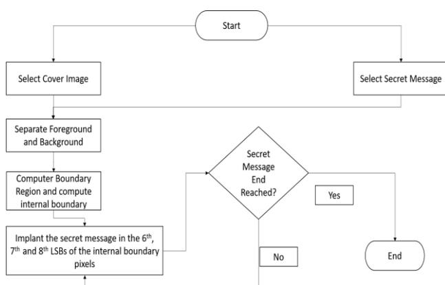
**Fig.2 Workflow of Embedding algorithm**
