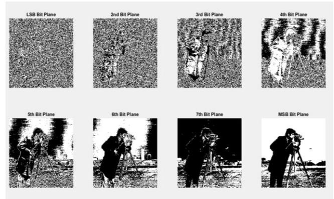
Fig.1 Bit Plane Slicing
