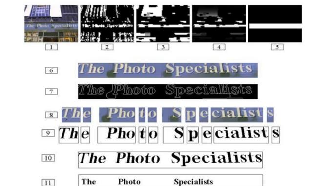
Fig. 2. Text detection (1, 2, 3, 4, 5), extraction (6, 7, 8, 9, 10), recognition (11), translation and transcription [25]
