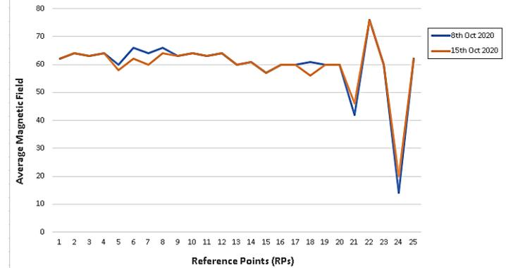
Fig. 1. Distribution of magnetic field in an empty room in the building on two different days.
